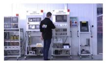
We have test stands developed by us, thanks to which we check whether the device is operational. They make sure that SEW EURODRIVE 822675X.13.16 is repaired.
